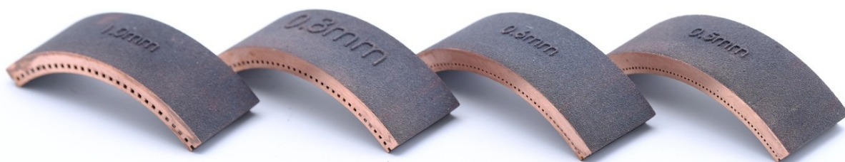
Figure 3: The CuCrZr test pieces for channel hole sizes for 1.0mm, 0.8mm, 0.6mm and 0.5mm.
