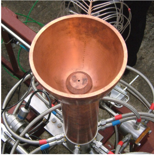
Figure 1: Stern 5kN rocket engine with an expansion-deflection nozzle
