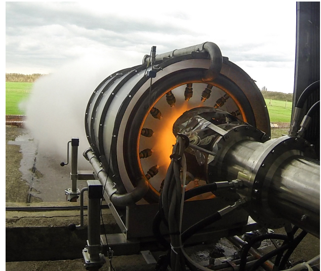
(b) Firing with water-spray sound suppression
