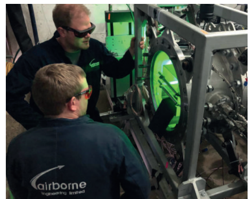
Laser instrumentation on a combustion test rig
