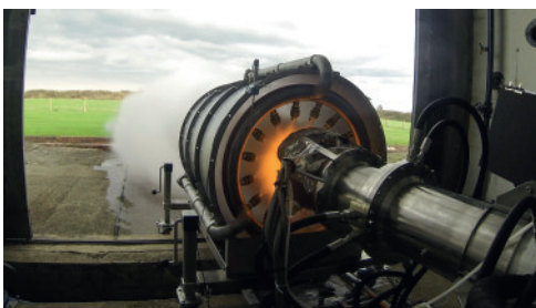
STOIC engine firing with water sound suppression
