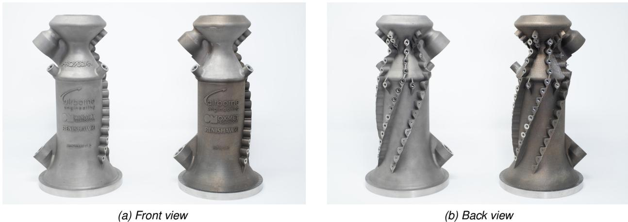
Figure 4: First combustion chamber test pieces (v1.0) with ABD<sup>®</sup>-900AM on the left and IN718 on the right.
