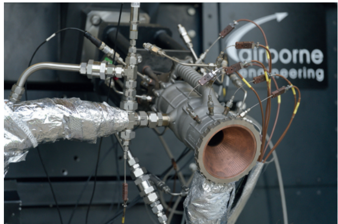
A custom-designed dual-cooled LOX/LCH4 engine additively manufactured from GRCop-42/Inconel-718 to support an ESA research programme
